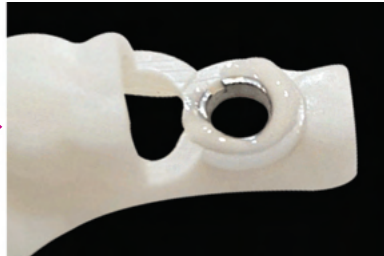
[Figure. 2] Bond the metal ring with resin cement
